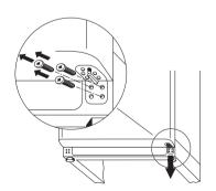
4. Move the bearing pivot from the right to the left hand hole. Remove the freezer compartment door carefully to the front and place on one side.
